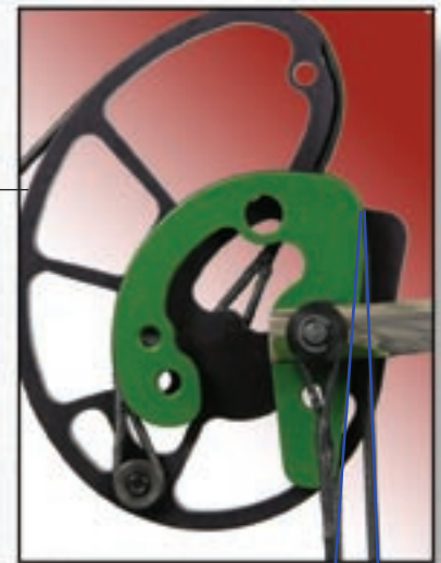
At full draw both cams should have the buss cable parallel to the back of the base cam as in figure 1.
