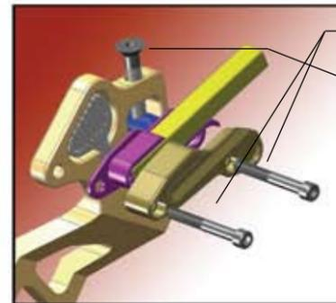
Start by loosening the 2 pocket clamping bolts, one full turn only. Once these bolts are loose you can adjust the peak weight.
