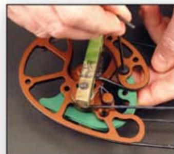
Once you have changed the draw module, re-place the screw and tighten. Draw Modules are available in 1/2 inch increments.
