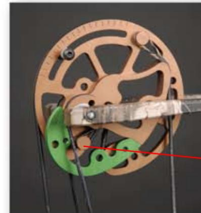
The gap on the bottom cam should always be 1/8" to 3/16" with the top cam set from 1/16" to 1/8". The important thing to remember is to always keep the post on the top cam around 1/16" closer to the yoke cable than the bottom cam.
