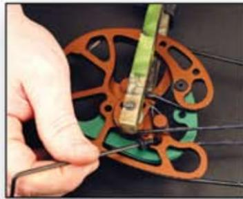
Start by removing the screws holding the draw module in place.
