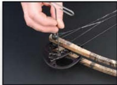
Start by removing the screw that is holding the draw module in place (the screw placement for your cam is pictured above).
